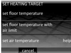
Your thermostat is capable of using a floor temperature sensor, air temperature sensor or both for thermal regulation. If you are using your floor heating as secondary heating source (such as in the bathroom) then you might prefer to use the floor temperature. However if the floor heating is the primary heating source in your home you might prefer to use the air temperature.
